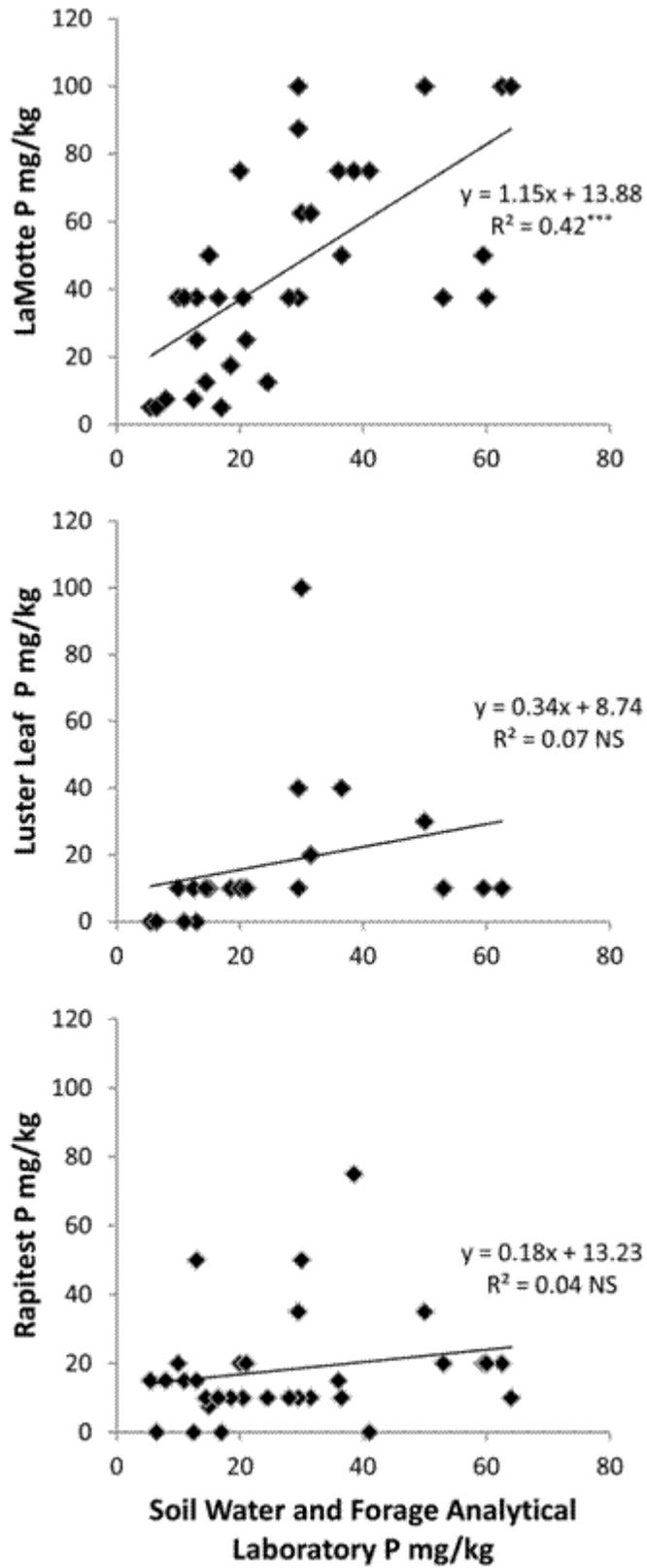
Figure 3. Comparison of soil test P using different test kits with standard laboratory practices.  $P=0.001$  ( $^{***}$ ), NS=not significant at 0.05 level.
