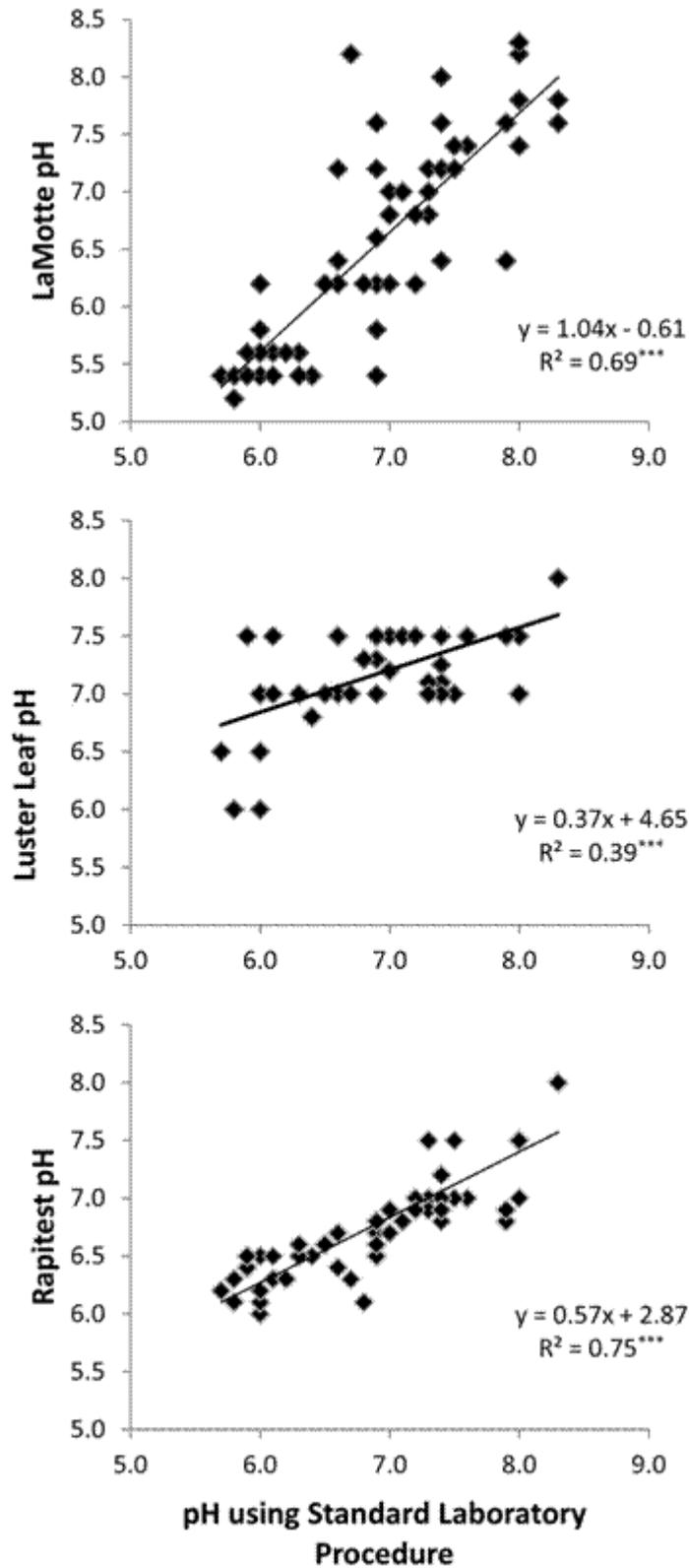
Figure 1. Comparison of soil pH using different test kits with standard laboratory practices.  $P=0.001$  (\*\*\*) , NS=not significant at 0.05 level.
