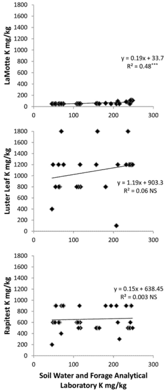
Figure 4. Comparison of soil test K using different test kits with standard laboratory practices.  $P=0.001$  ( $^{***}$ ), NS=not significant at 0.05 level.
