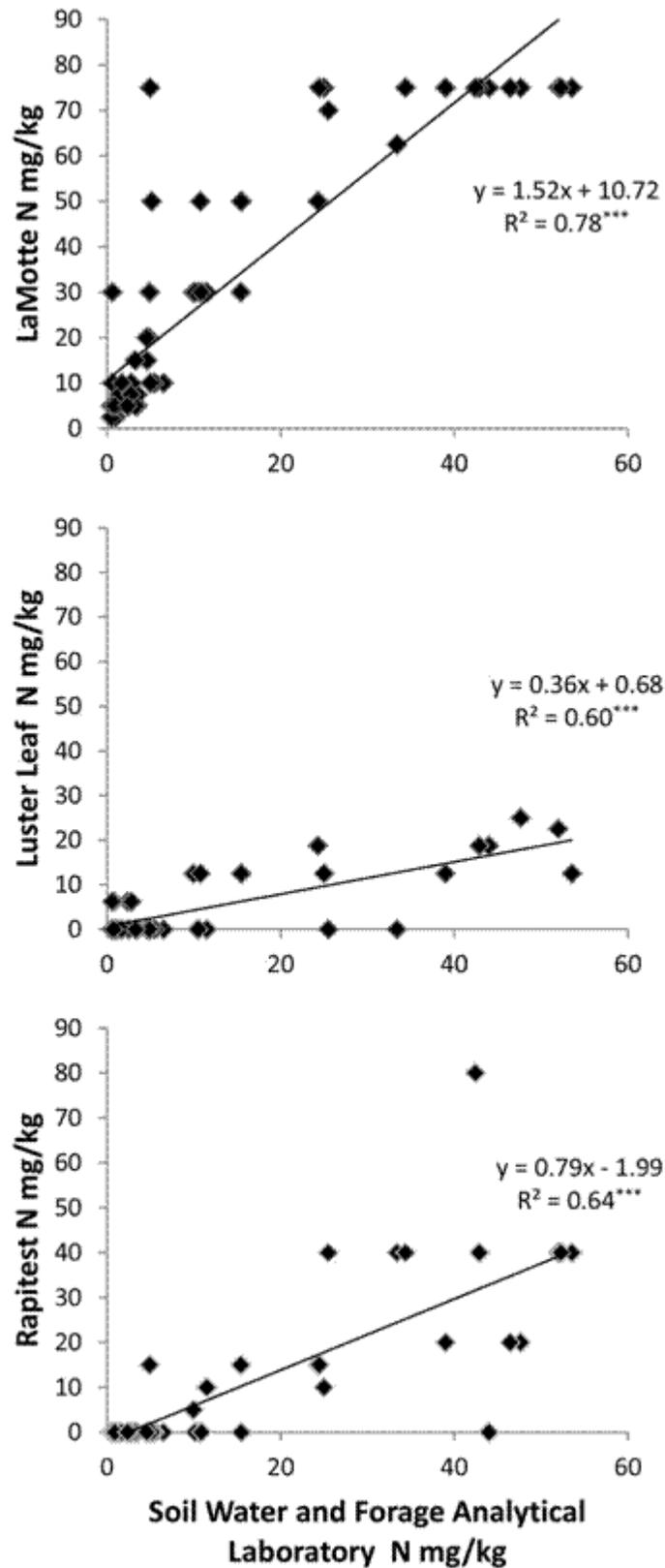
Figure 2. Comparison of soil N using different test kits with standard laboratory practices. P=0.001 (\*\*\*), NS=not significant at 0.05 level.
